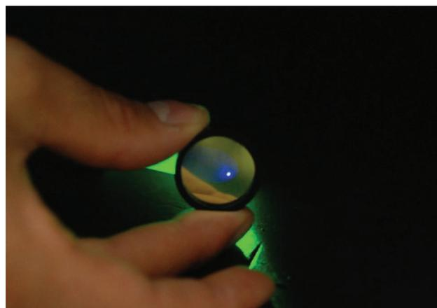
**Figure 4.** Upconversion of a dried sample of dyed nBA nanoparticles excited at 543 nm through a 500 nm short pass filter.
