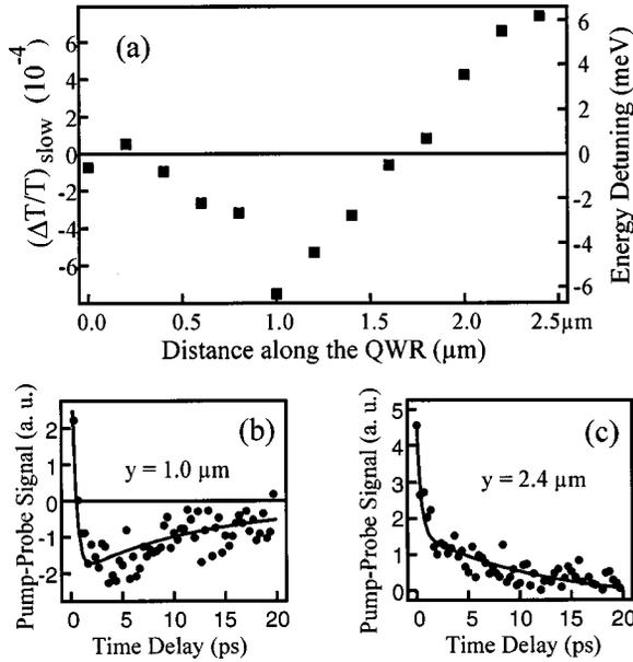
FIG. 3. (a) Amplitude  $(\Delta T/T)_{\text{slow}}$  of the slowly decaying contribution of near-field pump-probe traces vs position along a single QWR at fixed center laser photon energy of 1.578 eV. The right axis indicates the calculated energy detuning variation along the wire. (b) and (c) are pump-probe traces at two different positions, 1.0 and 2.4  $\mu\text{m}$ , respectively.
